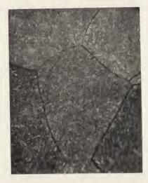
Fig. 34. (x 35 Diameters. Vertical Illumination.) Polished Section near base of Cu-Al Alloy. Shows granular structure.
